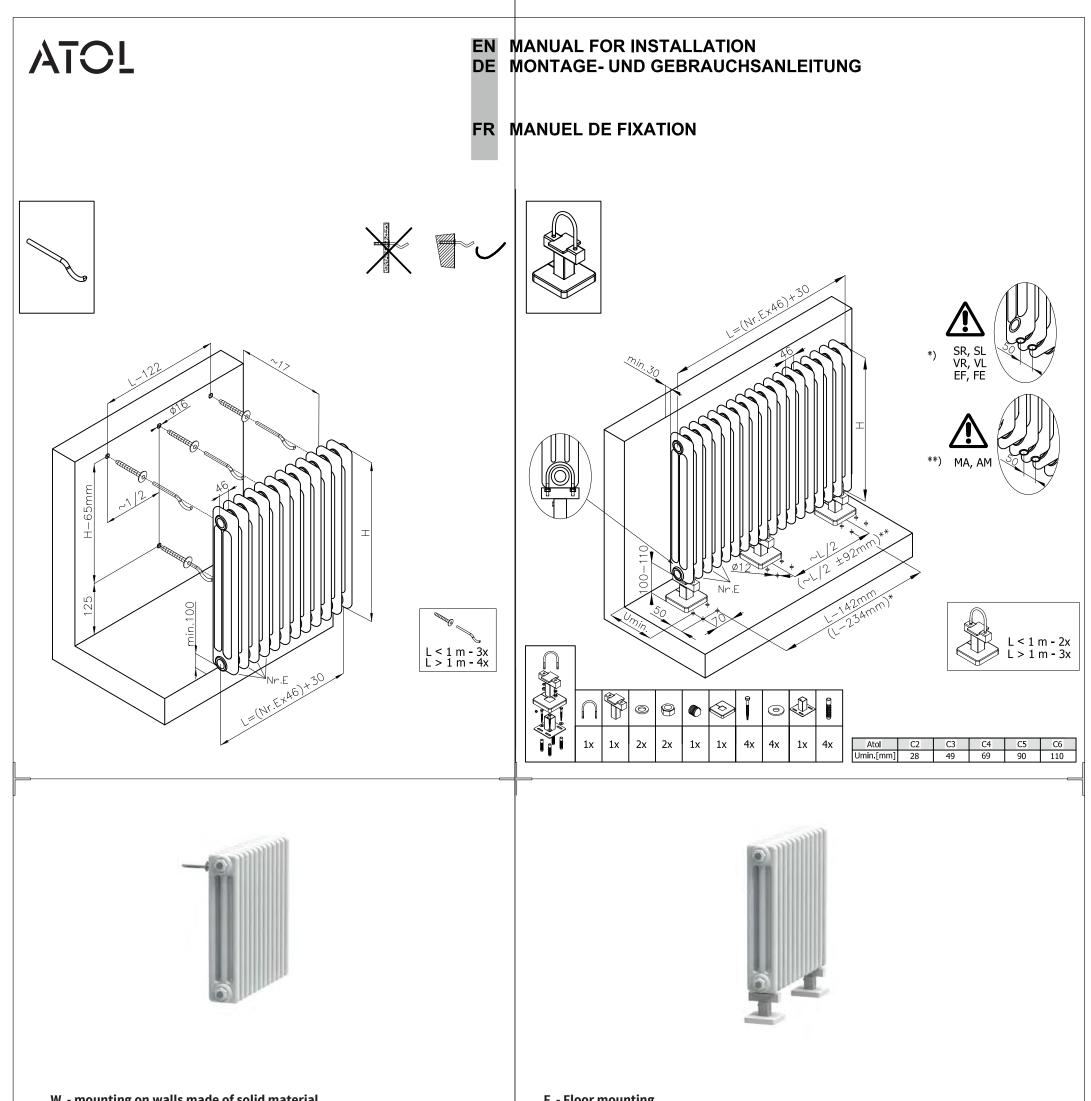
W - mounting on walls made of solid material Designed for mounting ATOL units on walls made of solid bricks, blocks or cast concrete. The wall must comply with the minimum thickness requirements.
