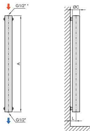
The unit does not have an air-vent valve, it is necessary to vent on the upper inlet pipe a) or use a single-point valve b)
