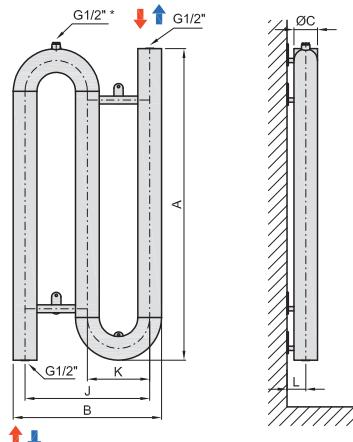
The unit does not have an air-vent valve on top inlet, it is necessary to vent on the inlet pipe
