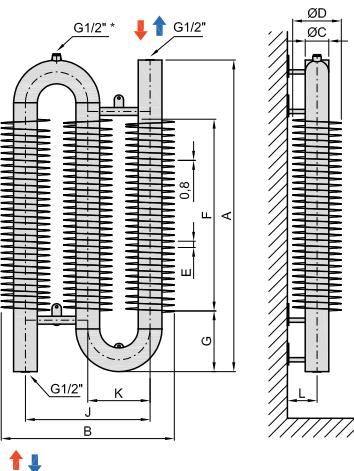
The unit does not have an air-vent valve on top inlet, it is necessary to vent on the inlet pipe
