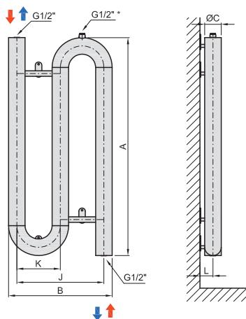
The unit does not have an air-vent valve on top inlet, it is necessary to vent on the inlet pipe
